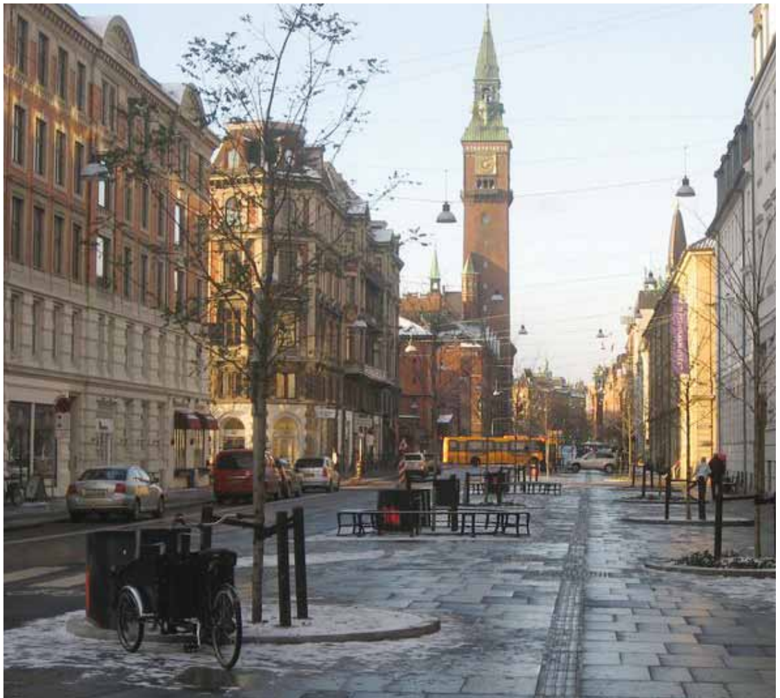
Metre-high black units installed during the winter months only to protect trees from the effects of salt spray on busy traffic routes. Image: Anne Jaluzot
