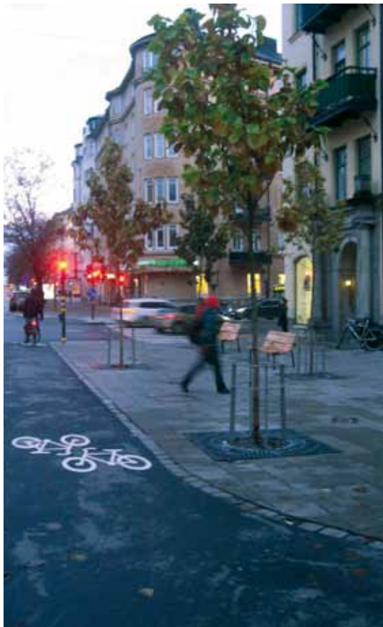
Low-level multipurpose protection in central Stockholm, Sweden.
