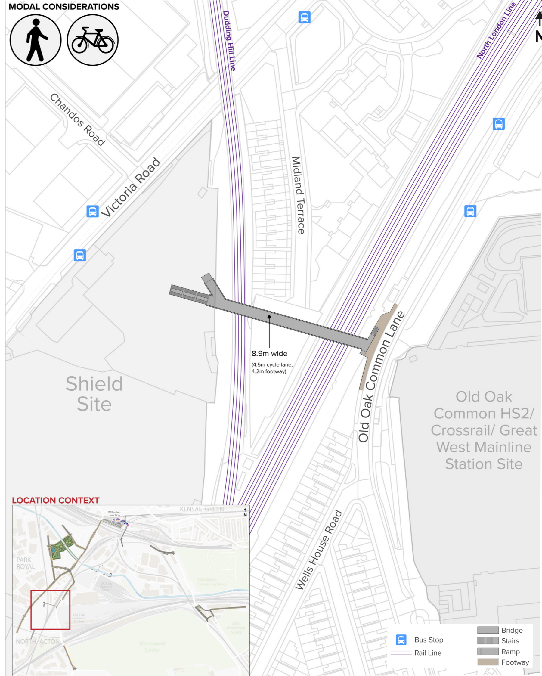
Figure 15: Intervention 2b, proposed layout for a new pedestrian and cycle bridge between the Shield Site and Old Oak Common Lane
