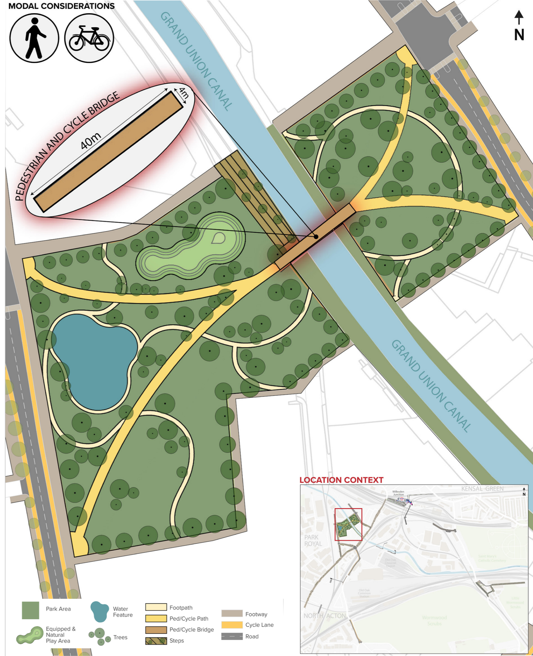
Figure 36: Intervention 6c, proposed design for pedestrian and cycle bridge over the Grand Union Canal
