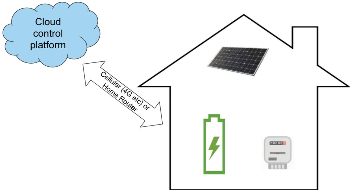
*Figure 4: Control architecture for remote ESS control*
