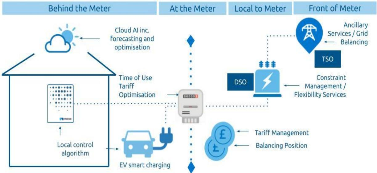
Figure 1 - System diagram explain battery relative to wider system
