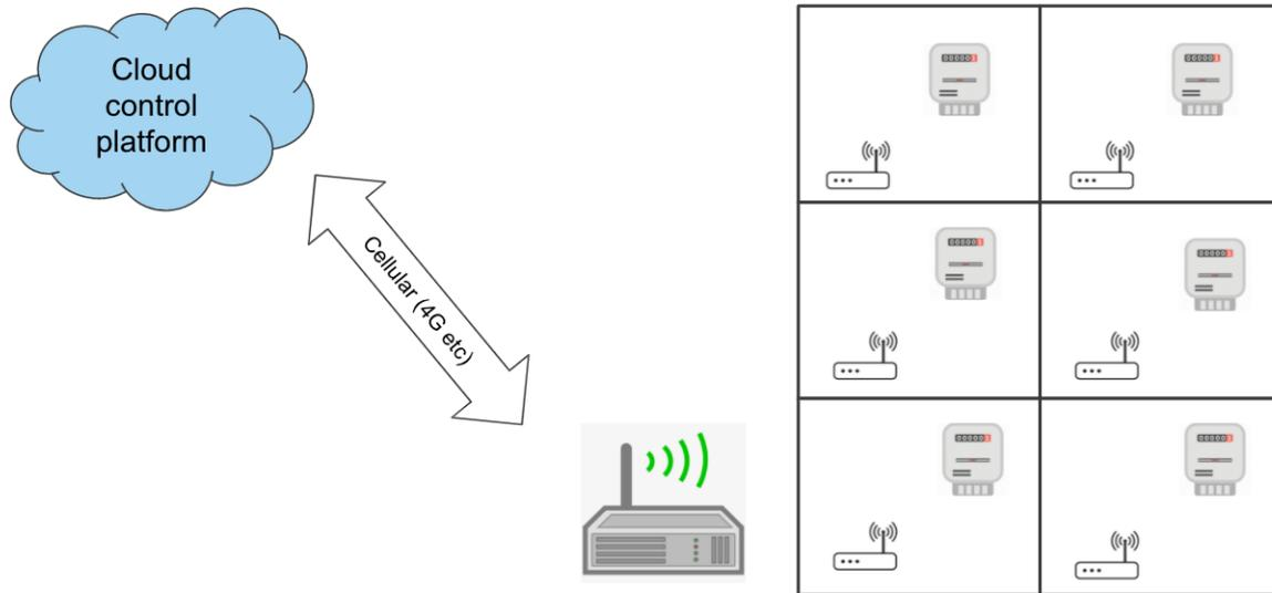
*Figure 8: Control scheme for a Mesh Network*
