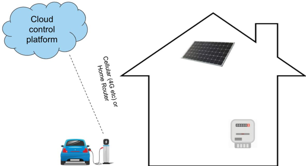
*Figure 6: Control architecture for remote (CPO type) electric vehicle charger control*
