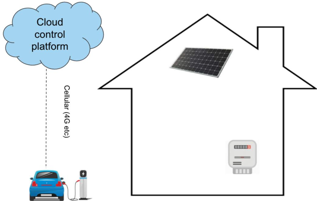
Figure 7: Control architecture for remote EV control
