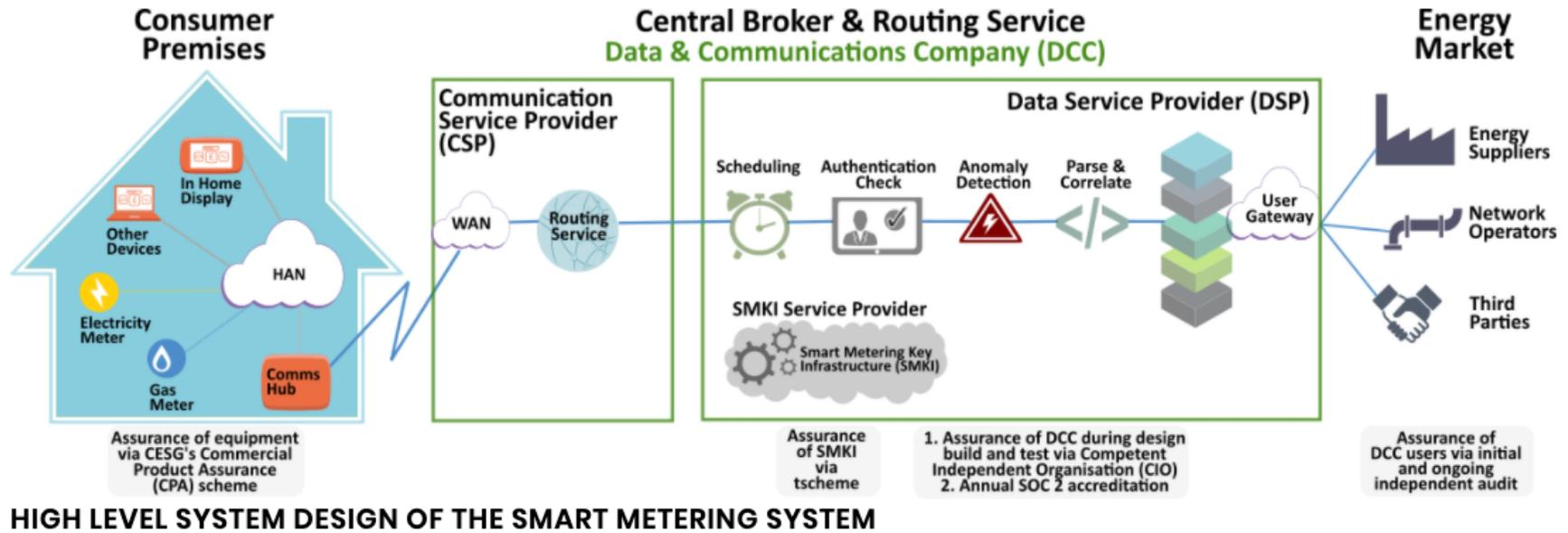
figure 10: DCC communication system schematic from ref;
