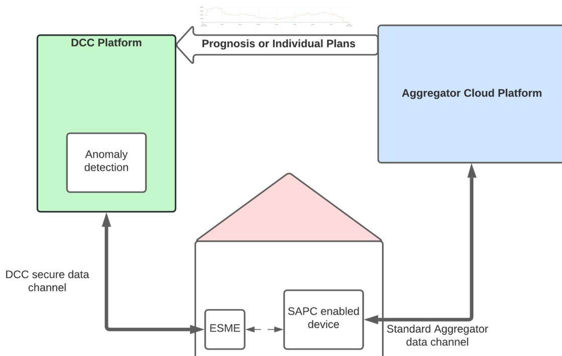
Figure 11: Simple diagram of architecture for proposal 1
