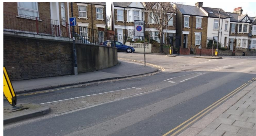
Figure 4-12: Steep gradients with crossfall (L19)
