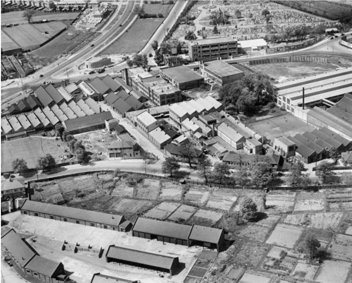
Figure 31: This oblique aerial photograph from a 1931 Aerofilms sortie shows a slice of industrial North Acton. The jumble of north light roofed structures between Wales Farm Road and Victoria Road include the Telegraph Condenser Works (Aerofilms' client), the Actona biscuit works, Victoria Paper Mills, a scientific instrument factory and a rubber works complete
