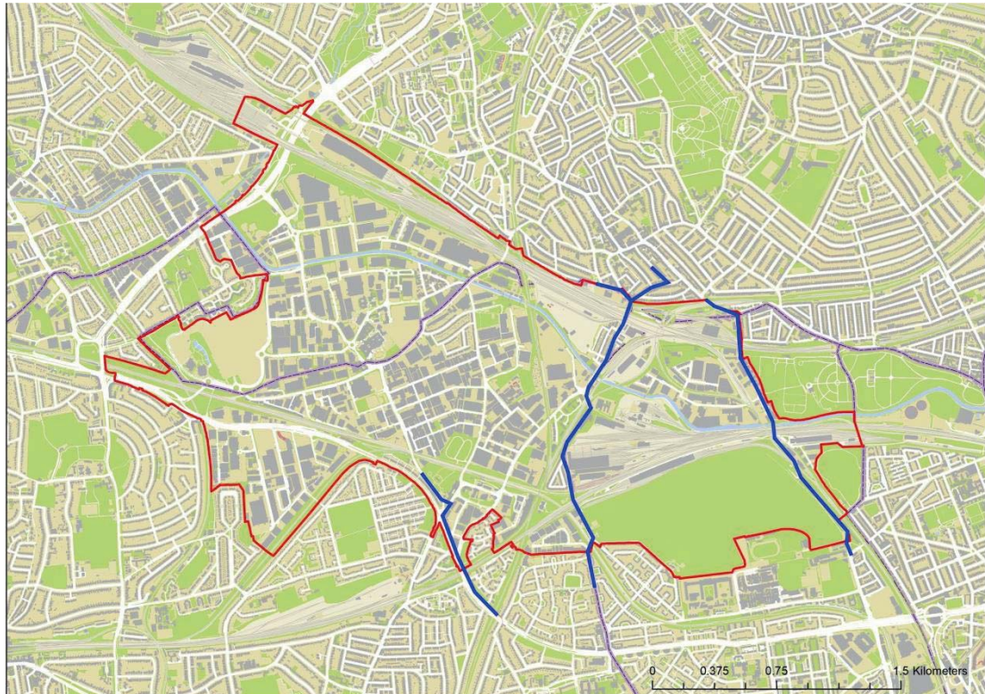
Figure 16.1 Existing potable water mains
