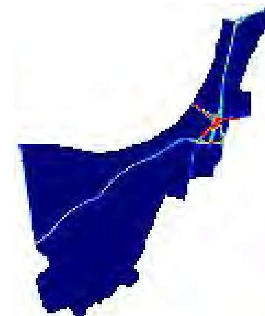
Figure 9.11 Modelled number of exceedences (days) above the daily mean PM 10 concentration using the LAEI 2004 emissions datasets and 2004 meteorology.
