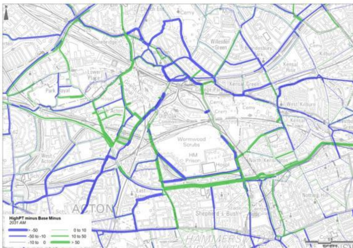
Figure 9-3: Traffic flows – Reduced Highway/ High PT Share scenario vs. 2031 Reference Case AM pk
