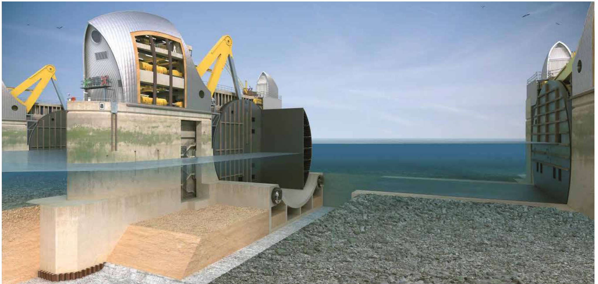
THAMES BARRIER GATE CUTAWAY IMAGE
