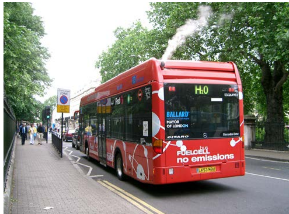
ZERO EMISSION HYDROGEN FUELCELL BUS IN LONDON. THE 'EXHAUST' SEEN HERE AT THE TOP OF THE VEHICLE IS ONLY PURE WATER VAPOUR.
