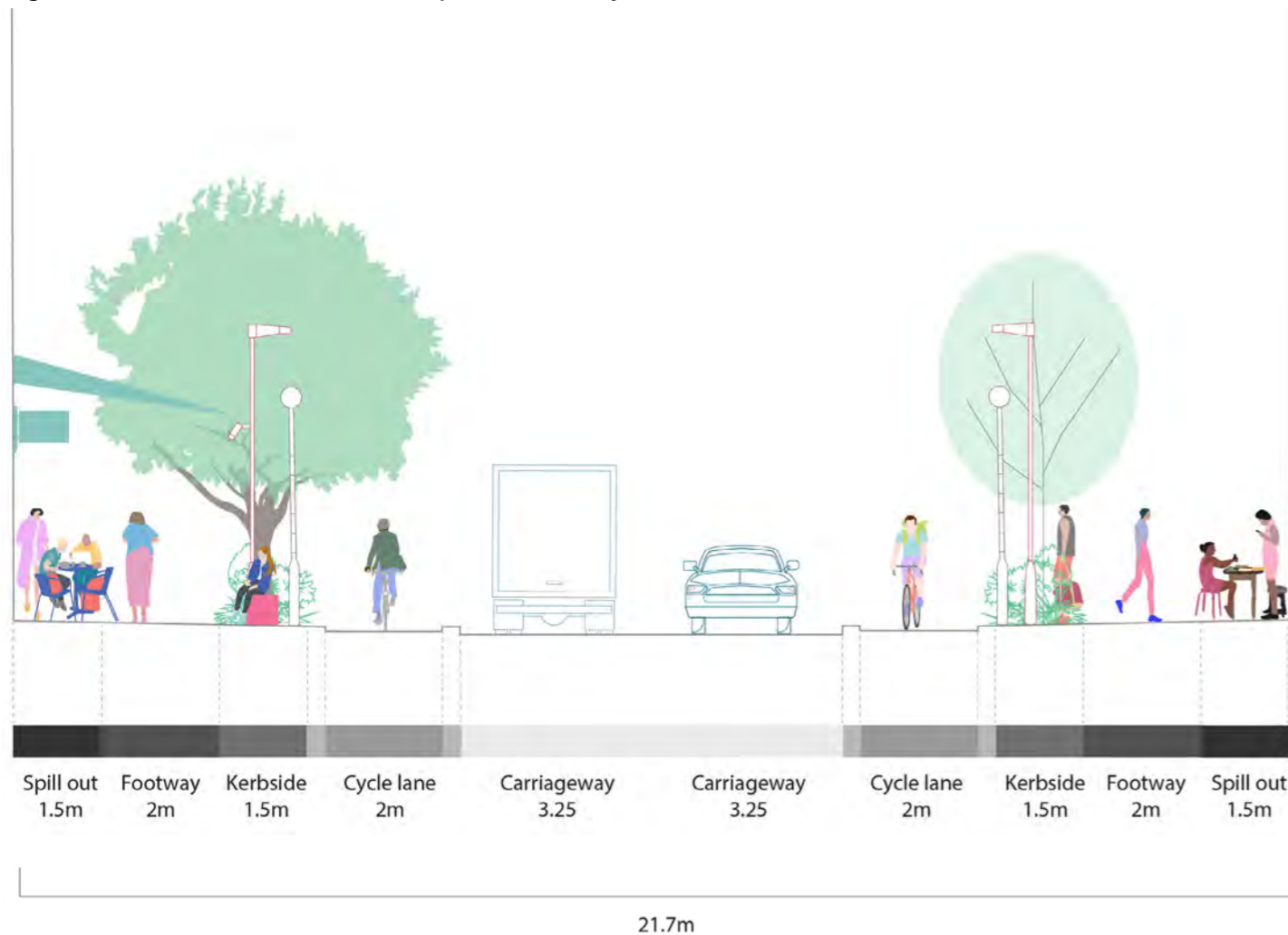
Figure 6.15 Illustration of an example Secondary Street street-section in a mixed use area
