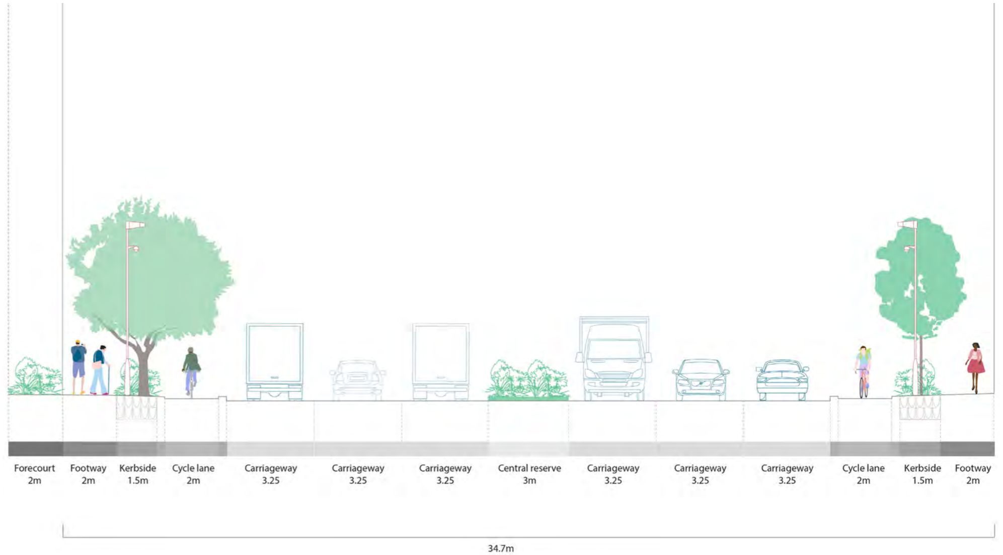
Figure 6.11 Illustration of an example Primary Street street-section
