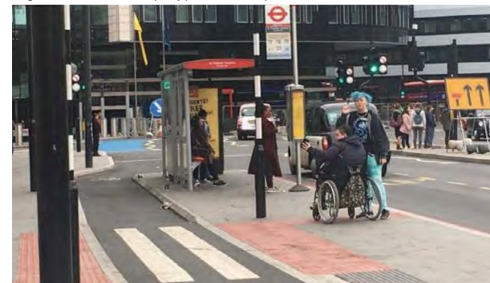
Figure 6.13 Bus stop bypass example, London
