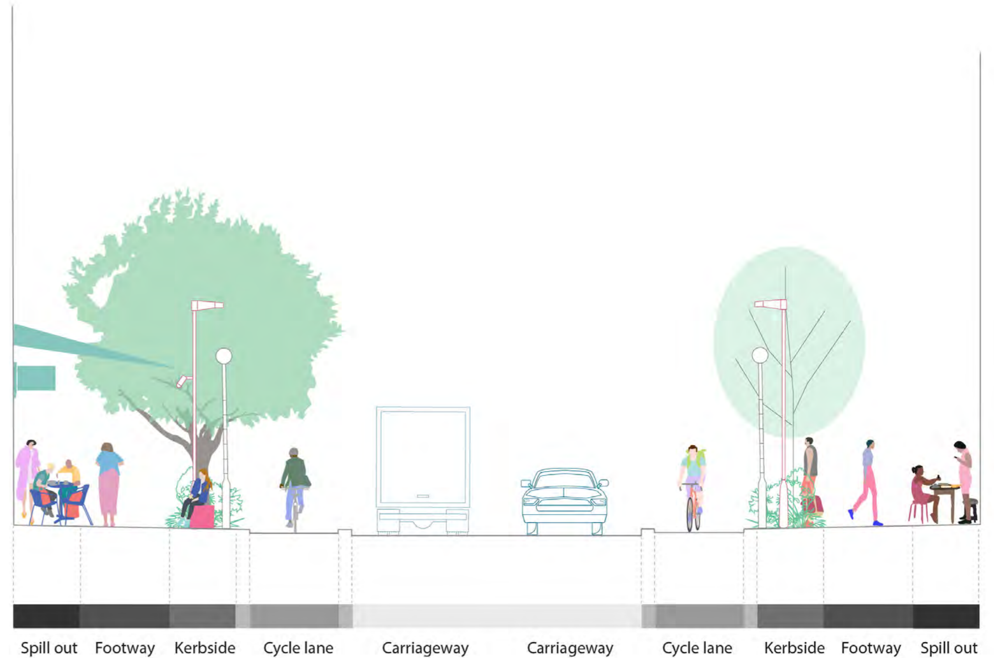
Figure 6.2 Illustration of potential street components
