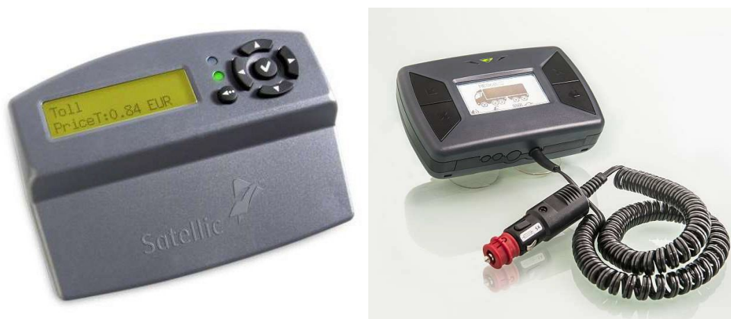
Figure 3: On-board devices used in Europe for HGV road user charging
