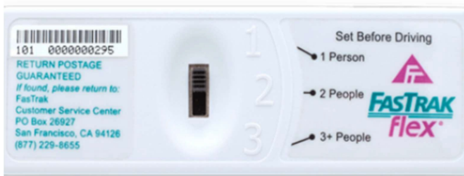
Figure 2: A Bay Area FasTrak toll tag for a high occupancy vehicle discount/exemption
