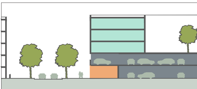
Mid-density mixed-use: retail parking can be at ground level or basement, with residential parking at first floor to provide easier access to flats above
