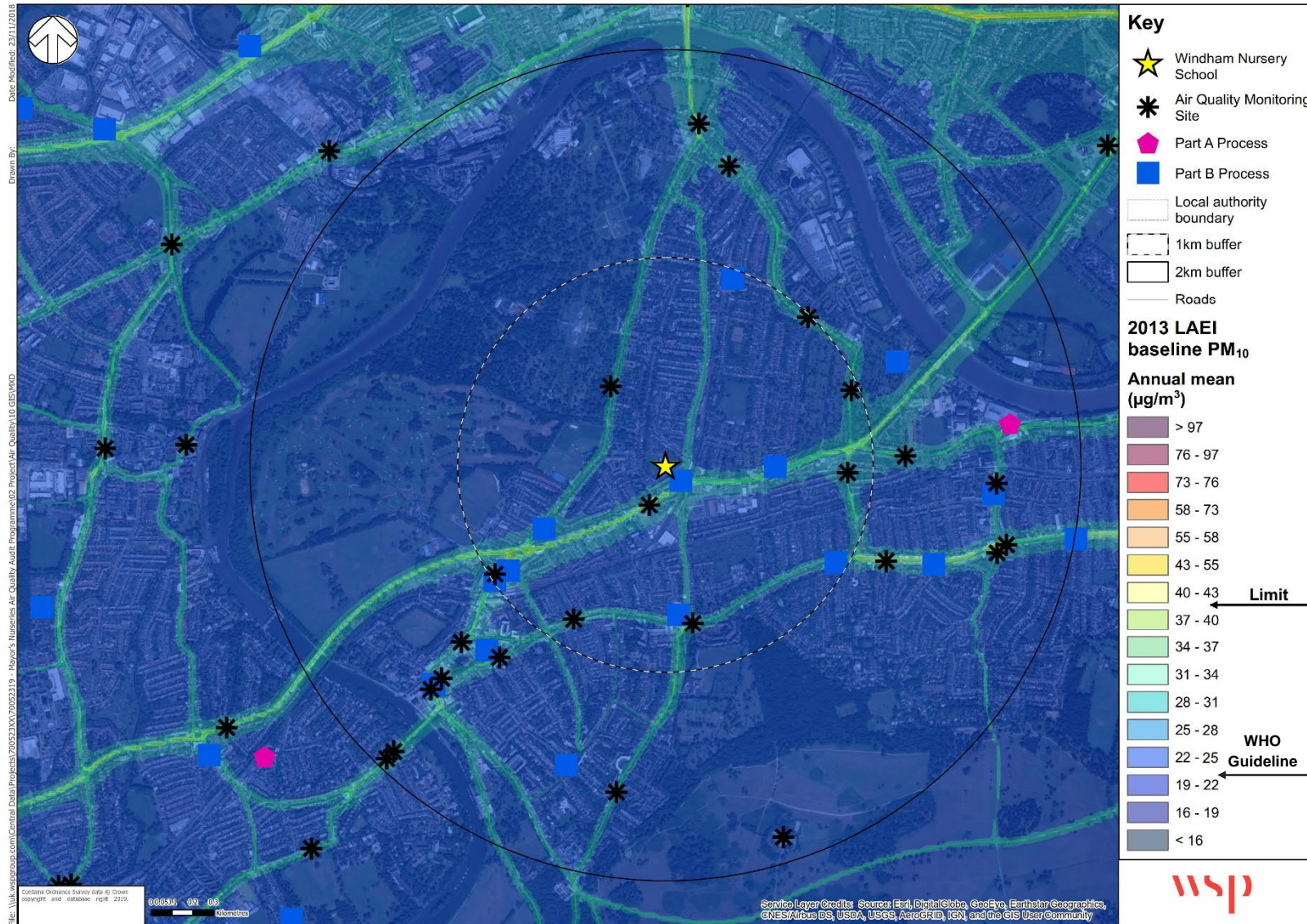
Figure 12 - 2013 LAEI Baseline Annual Mean PM 10 Concentrations within 2km of Windham Nursery School
