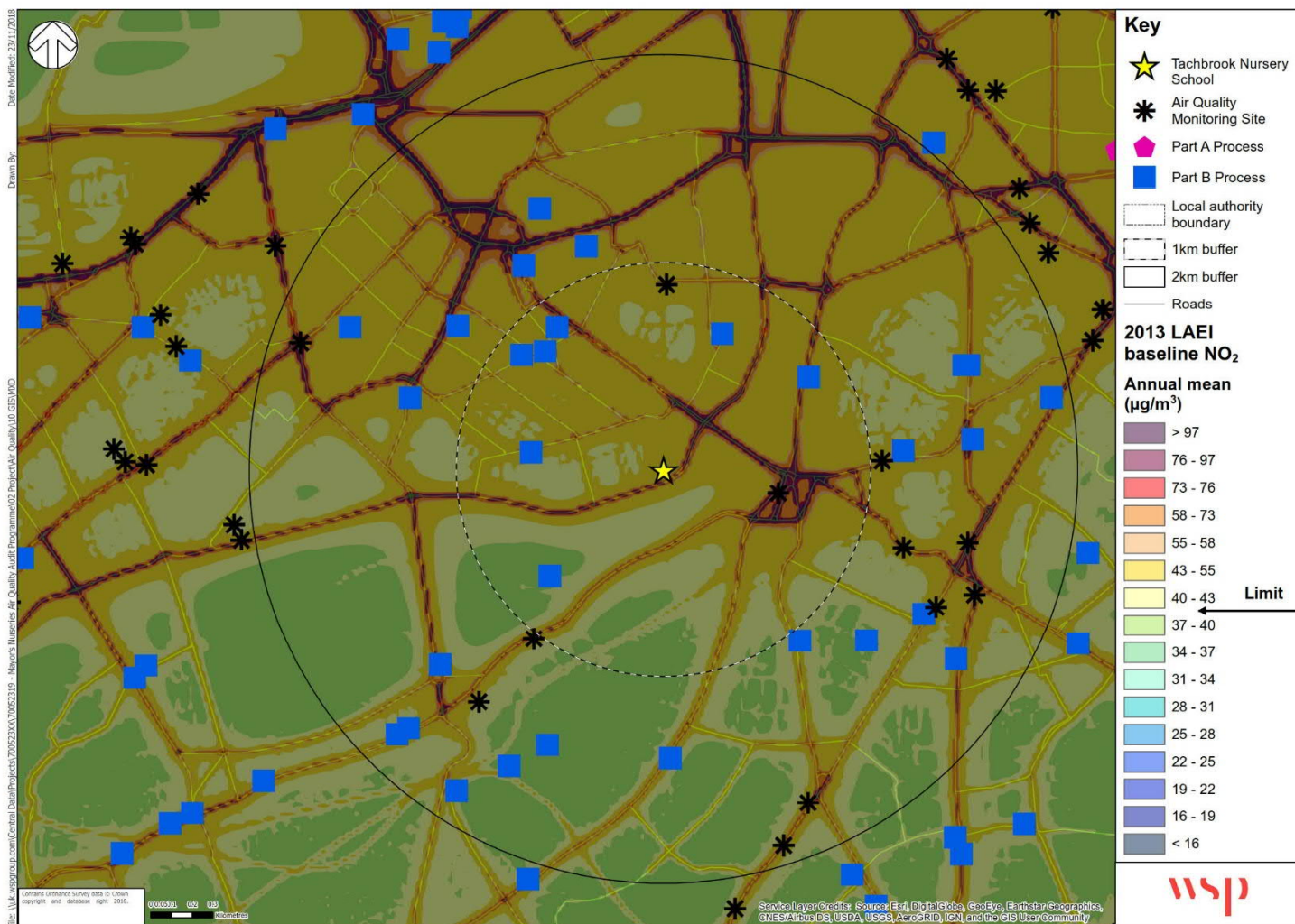
Figure 11 – 2013 LAEI Baseline Annual Mean NO 2 Concentrations within 2km of Tachbrook Nursery School
