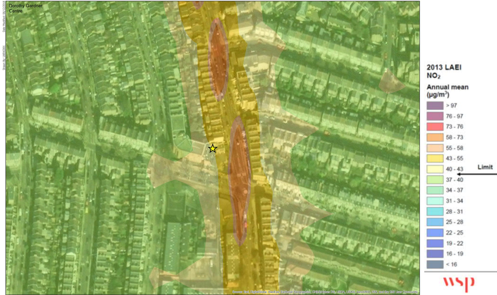
Figure 6 - LAEI Baseline Annual Mean NO 2 Concentrations within the Immediate Area of Dorothy Gardner Nursery School
