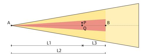
Diagram explaining variable used in ameded formula for the calculating the Curvature of the Earth compensation
