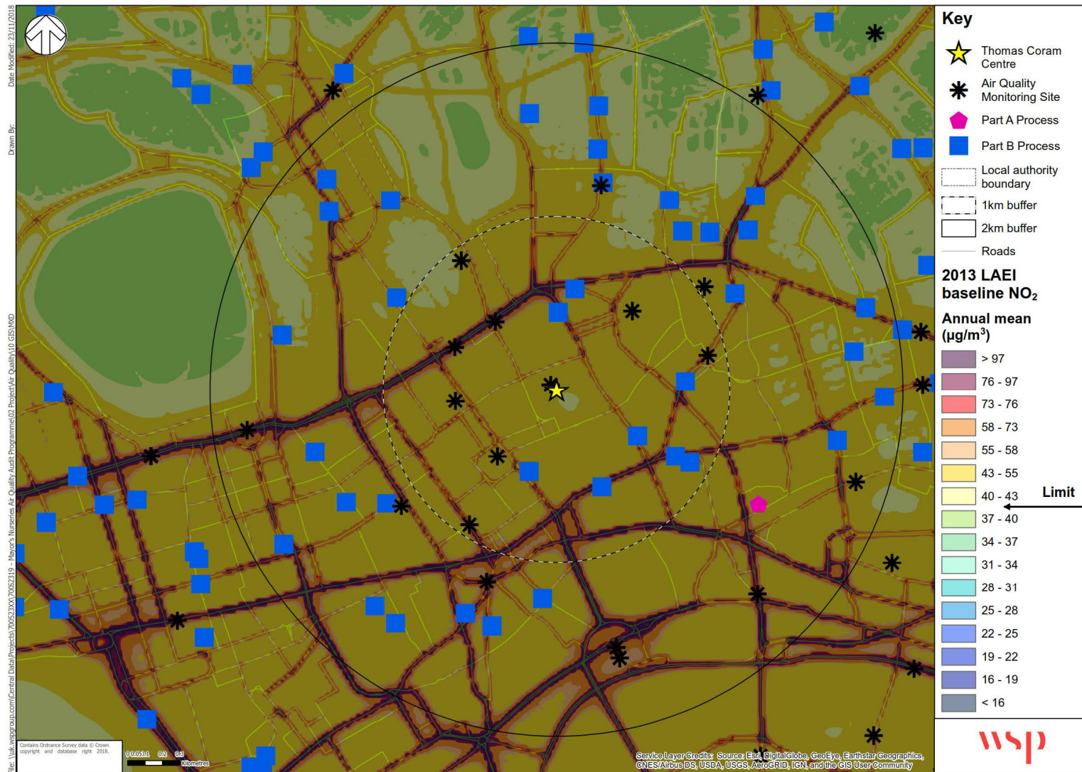
Figure 11 – 2013 LAEI Baseline Annual Mean NO 2 Concentrations within 2km of Thomas Coram Centre
