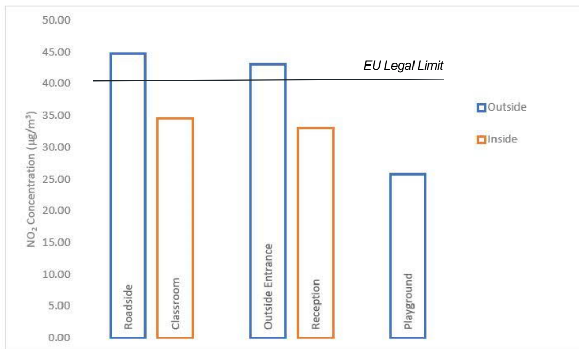
Figure 5 - Comparison of the average NO 2 concentrations at Columbia Market Nursery School (µg/m 3 )
