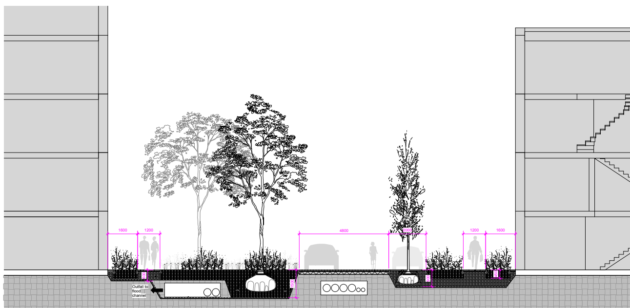
typical section through public realm, showing location attenuation alongside other below ground features.
