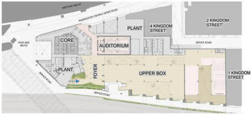
Figure 15: Schematic B2 floor plan.
