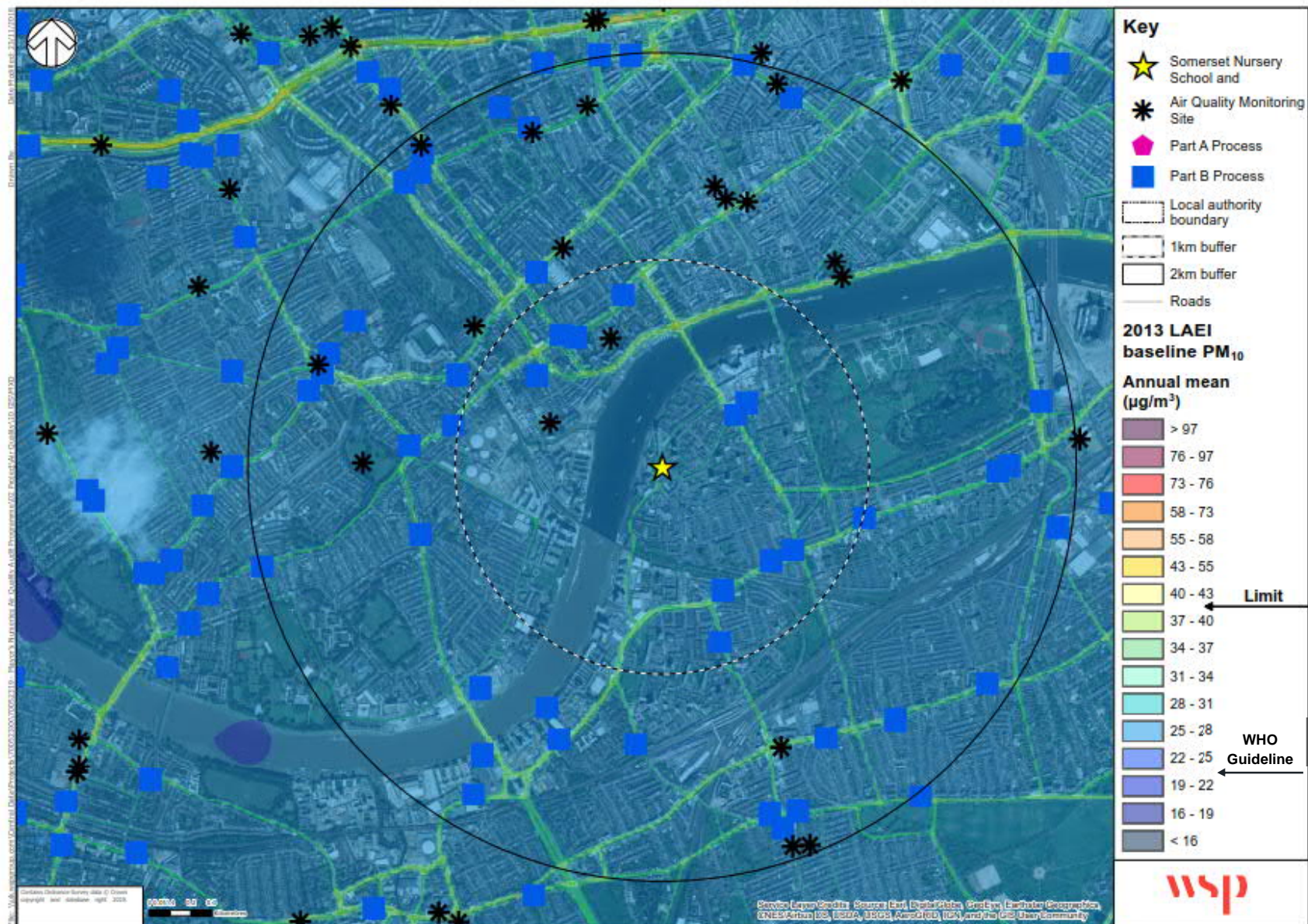
Figure 12 - 2013 LAEI Baseline Annual Mean PM 10 Concentrations within 2km of Somerset Nursery School and Children's Centre
