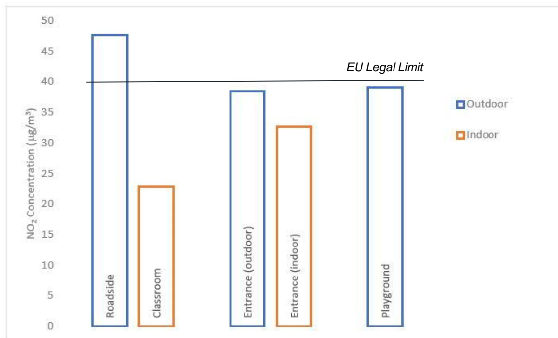
Figure 5 - Comparison of the average NO 2 concentrations at Alice Model Nursery School (µg/m 3 )
